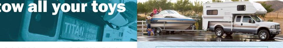
When towing behind a Lance camper, extending the hitch from the truck rearward to the camper bumper is necessary.
